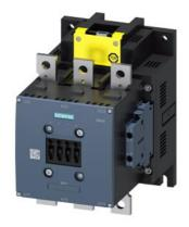
power contactor, AC-3e/AC-3 265 A, 132 kW / 400 V AC (50-60 Hz) / DC 96-127 V x (0.8-1.1) F-PLC input 24 V DC 3-pole, auxiliary contacts 2 NO + 2 NC drive: electronic main circuit: busbar control and auxiliary circuit: screw terminal
