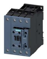
contactor AC-1, 110 A, 400 V / 40 °C, 4-pole, 220 V AC, 50 Hz / 240 V, 60 Hz, auxiliary contacts: 1 NO + 1 NC, screw terminal, size: S2
