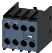
auxiliary switch, on the front, 2 NC, .1/.2, .1/.2, --/--, current path: 1 NC, 1 NC, --, --, screw terminal, for contactors 3RT2 and contactor relays 3RH2
