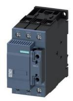
capacitor contactor, AC-6b 50 kVAr, / 400 V, 3-pole, 110 V AC, 50 Hz / 120 V, 60 Hz, auxiliary contacts: 2 NC, screw terminal, size: S2  $\,$
