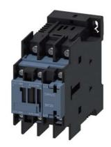
power contactor, AC-3e/AC-3, 25 A, 11 kW / 400 V, 3-pole, 24 V DC, auxiliary contacts: 1 NO + 1 NC, ring cable lug connection, size: S0  $\,$
