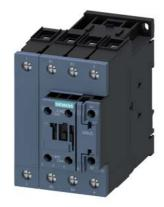
power contactor, AC-3, 51 A, 22 kW / 400 V, 4-pole, 175-280 V AC/DC, 50/60 Hz, with integrated varistor, main contacts: 2 NO + 2 NC, auxiliary contacts: 1 NO + 1 NC, screw terminal, size: S2
