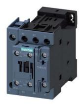
power contactor, AC-3, 25 A, 11 kW / 400 V, 4-pole, 24 V DC, main contacts: 2 NO + 2 NC, auxiliary contacts: 1 NO + 1 NC, screw terminal, size: S0
