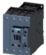
contactor AC-1, 110 A, 400 V / 40  $^\circ$ C, 4-pole, 230 V AC, 50 Hz, auxiliary contacts: 1 NO + 1 NC, screw terminal, size: S2
