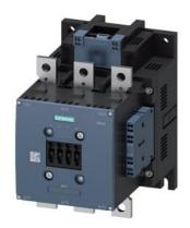
power contactor, AC-3e/AC-3 300 A, 160 kW / 400 V, AC (50-60 Hz) / DC Uc: 21-27, 3 V PLC input 24 V DC 3-pole, auxiliary contacts 2 NO + 2 NC drive: electronic main circuit: busbar control and auxiliary circuit: spring-loaded terminal
