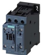
power contactor, AC-3e/AC-3, 12 A, 5.5 kW / 400 V, 3-pole, 24 V DC, auxiliary contacts: 1 NO + 1 NC, screw terminal, size: S0, communication-capable
