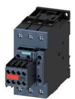
power contactor, AC-3e/AC-3, 80 A, 37 kW / 400 V, 3-pole, 24 V DC, 0.8-1.2\* Us, with integrated varistor, auxiliary contacts: 2 NO + 2 NC, screw terminal, size: S2, suitable for PLC outputs, captive auxiliary switch
