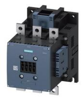
power contactor, AC-3e/AC-3 300 A, 160 kW / 400 V, AC (50-60 Hz) / DC Uc: 23-26 V 3-pole, auxiliary contacts 2 NO + 2 NC drive: conventional main circuit: busbar control and auxiliary circuit: spring-loaded terminal
