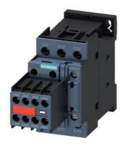
power contactor, AC-3e/AC-3, 38 A, 18.5 kW / 400 V, 3-pole, 110 V AC, 50 Hz / 120 V, 60 Hz, with plugged-in varistor, auxiliary contacts: 2 NO + 2 NC, screw terminal, size: S0, captive auxiliary switch
