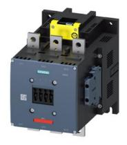
power contactor, AC-3e/AC-3 500 A, 250 kW / 400 V AC (50-60 Hz) / DC 200-277 V x (0.8-1.1) F-PLC input 24 V DC 3-pole, auxiliary contacts 2 NO + 2 NC permanently mounted drive: electronic main circuit: busbar control and auxiliary circuit: screw terminal
