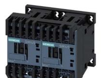
reversing contactor assembly, AC-3e/AC-3, 7 A, 3 kW / 400 V, 3-pole, 110 V AC, 50 Hz / 120 V, 60 Hz, spring-loaded terminal, electrical and mechanical interlock
