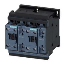
reversing contactor assembly, AC-3e/AC-3, 25 A, 11 kW / 400 V, 3-pole, 110 V AC, 50/60 Hz, screw terminal, electrical and mechanical interlock, auxiliary contacts: 2 x 1 NO
