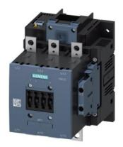
power contactor AC-1 275 A / 690 V / 40  $^{\circ}$ C 3-pole, Uc: 96-127 V AC(50-60 Hz) / DC PLC input 24 V DC drive: electronic auxiliary contacts 2 NO + 2 NC main circuit: busbar control and auxiliary circuit: screw terminal
