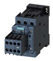
power contactor, AC-3e/AC-3, 17 A, 7.5 kW / 400 V, 3-pole, 110 V DC, auxiliary contacts: 2 NO + 2 NC, screw terminal, size: S0, removable auxiliary switch
