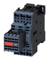
power contactor, AC-3e/AC-3, 17 A, 7.5 kW / 400 V, 3-pole, 24 V DC, with plugged-in diode combination, auxiliary contacts: 2 NO + 2 NC, spring-loaded terminal, size: S0, captive auxiliary switch
