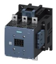
power contactor, AC-3e/AC-3 500 A, 250 kW / 400 V AC (50-60 Hz) / DC Uc: 110-127 V 3-pole, auxiliary contacts 2 NO + 2 NC drive: conventional main circuit: busbar control and auxiliary circuit: spring-loaded terminal
