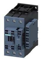
power contactor, AC-3e/AC-3, 65 A, 30 kW / 400 V, 3-pole, 110 V AC, 60 Hz, auxiliary contacts: 2 NO + 2 NC, main circuit: screw terminal, control and auxiliary circuit: spring-loaded terminal, size: S2, lateral auxiliary switch
