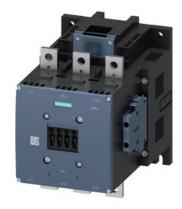
Power contactor, AC-3 500 A, 250 kW / 400 V AC (50-60 Hz) / DC 23-26 V AC / DC Auxiliary contacts 2 NO + 2 NC 3-pole, size S12 Busbar connections Operating mechanism: conventional screw terminals NEMA version
