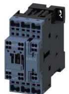
power contactor, AC-3e/AC-3, 38 A, 18.5 kW / 400 V, 3-pole, 24 V DC, auxiliary contacts: 1 NO + 1 NC, spring-loaded terminal, size: S0, communication-capable
