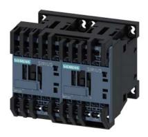
reversing contactor assembly, AC-3e/AC-3, 7 A, 3 kW / 400 V, 3-pole, 24 V AC, 50/60 Hz, spring-loaded terminal, electrical and mechanical interlock
