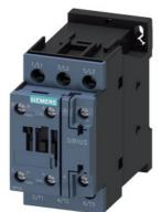
power contactor, AC-3e/AC-3, 38 A, 18.5 kW / 400 V, 3-pole, 208 V AC, 50/60 Hz, auxiliary contacts: 1 NO + 1 NC, screw terminal, size: S0
