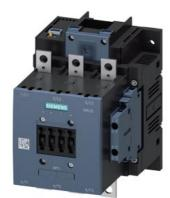
power contactor, AC-3e/AC-3 185 A, 90 kW / 400 V Uc: 24 V DC x (0.7-1.25) PLC input 24-110 V DC 3-pole, auxiliary contacts 2 NO + 2 NC drive: electronic main circuit: busbar control and auxiliary circuit: screw terminal extended rated condition railroad IEC 60077
