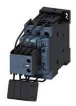
capacitor contactor, AC-6b 20 kVAr, / 400 V, 3-pole, 24 V DC, auxiliary contacts: 1 NO + 2 NC, screw terminal, size: S0  $\,$
