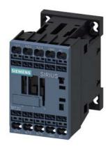
power contactor, AC-3e/AC-3, 12 A, 5.5 kW / 400 V, 3-pole, 24 V AC, 50/60 Hz, auxiliary contacts: 1 NO, spring-loaded terminal, size: S00
