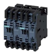
reversing contactor assembly, AC-3e/AC-3, 12 A, 5.5 kW / 400 V, 3-pole, 24 V DC, spring-loaded terminal, electrical and mechanical interlock, auxiliary contacts:  $2\times1$  NO
