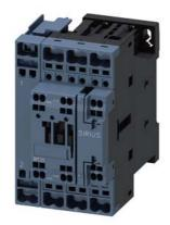
power contactor, AC-3, 25 A, 11 kW / 400 V, 4-pole, 110 V AC, 50 Hz, main contacts: 2 NO + 2 NC, auxiliary contacts: 1 NO + 1 NC, spring-loaded terminal, size: S0
