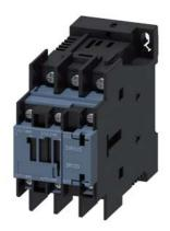
power contactor, AC-3e/AC-3, 17 A, 7.5 kW / 400 V, 3-pole, 24 V DC, 0.7-1.25\* Us, with plugged-in varistor, auxiliary contacts: 1 NO + 1 NC, ring cable lug connection, size: S0, suitable for PLC outputs, not expandable with auxiliary switch
