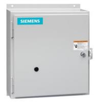
Mechanically held lighting contactor, Contactor amp rating 20A, 0 N.C. / 4 N.O. poles, Non-combination type, Enclosure NEMA type 12, Dust/drip proof for indoors
