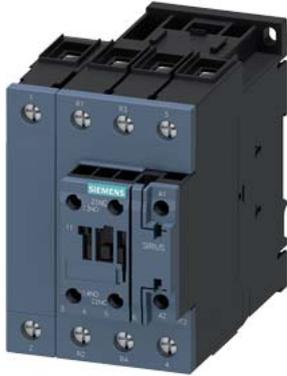
power contactor, AC-3, 40 A, 18.5 kW / 400 V, 4-pole, 110 V AC, 50 Hz, main contacts: 2 NO + 2 NC, auxiliary contacts: 1 NO + 1 NC, screw terminal, size: S2
