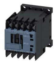
power contactor, AC-3e/AC-3, 16 A, 7.5 kW / 400 V, 3-pole, 24 V DC, auxiliary contacts: 1 NO, ring cable lug connection, size: S00  $\,$
