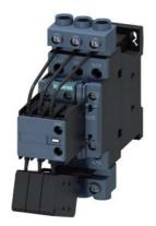
capacitor contactor, AC-6b 33 kVAr, / 400 V, 3-pole, 220 V AC, 50 Hz / 240 V, 60 Hz, auxiliary contacts: 1 NO + 2 NC, screw terminal, size: S0
