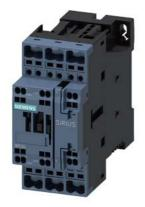
power contactor, AC-3e/AC-3, 25 A, 11 kW / 400 V, 3-pole, 200-280 V AC/DC, 50/60 Hz, with integrated varistor, auxiliary contacts: 1 NO + 1 NC, spring-loaded terminal, size: S0
