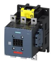
power contactor AC-1 400 A / 690 V / 40  $^{\circ}$ C 3-pole, Uc: 96-127 V AC(50-60 Hz) / DC F-PLC input 24 V DC drive: electronic auxiliary contacts 2 NO + 2 NC main circuit: busbar control and auxiliary circuit: screw terminal
