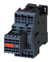
power contactor, AC-3e/AC-3, 38 A, 18.5 kW / 400 V, 3-pole, 24 V DC, auxiliary contacts: 2 NO + 2 NC, spring-loaded terminal, size: S0, captive auxiliary switch, no surge suppressor retrofittable
