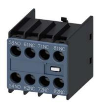
auxiliary switch, on the front, 1 NO + 3 NC, 53/54, 61/62, 71/72, 81/82, current path: 1 NO, 1 NC, 1 NC, 1 NC, screw terminal, physically coded, only with contactor relays 3RH2140 and 3RH2440 combinable (according to EN 50011)
