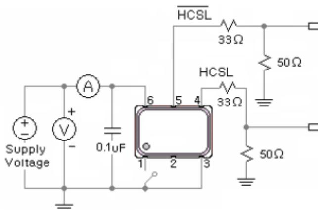
Note 12: Recommended test circuit images are representative of when the OE Function is located on Pin 1; when the OE Function is located on Pin 2, then Pin 1=No Connect & Pin 2=OE or No Connect.
