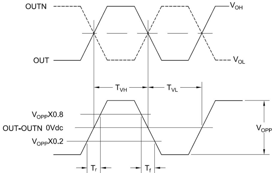
$$\text{Duty} = \frac{T_{VH}}{T_{VH} + T_{VL}} \times 100\%$$
