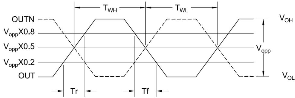
$$\text{Duty Cycle} = \frac{T_{WH}}{T_{WH} + T_{WL}} \times 100\%$$
