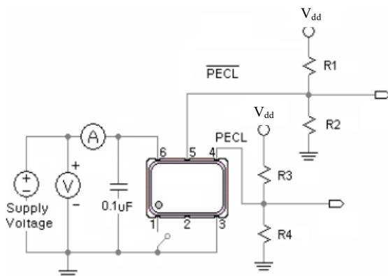
V<sub>dd</sub> = 3.3V; R<sub>1</sub>=R<sub>3</sub>=127Ω; R<sub>2</sub>=R<sub>4</sub>=82.5Ω
