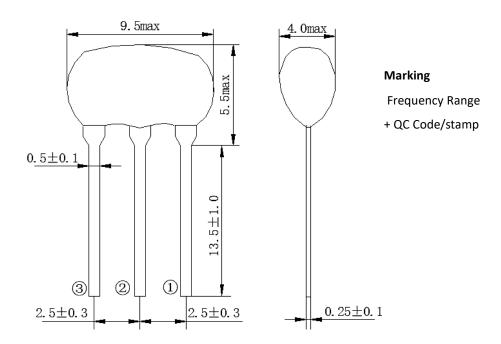
Connection: 1 Input 2 Ground 3 Output
