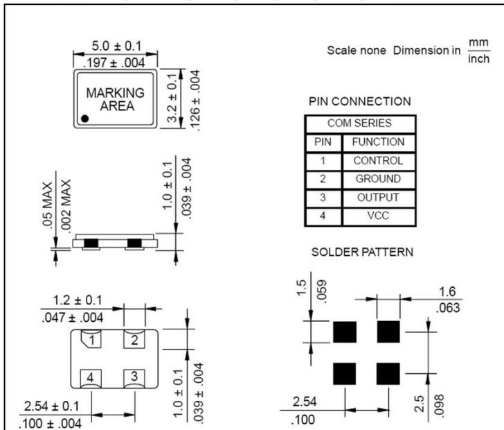
NOTE: A capacitor of 0.01  $\mu\text{F}$  between Vcc and Ground is recommended
