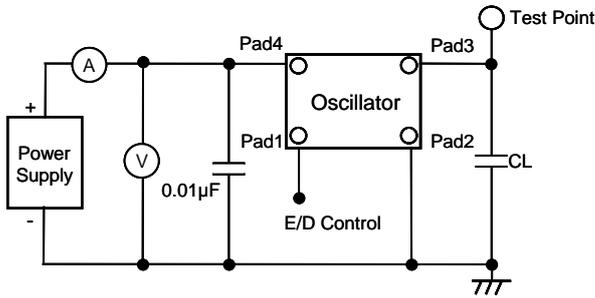
Note: CL includes probe and test fixture capacitance
