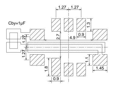
Note) Please connect the bypass capacitor (for example: 1 uF) of a power supply near the  $V_{CC}$  terminal.
