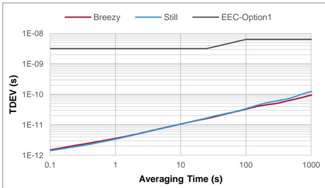
Figure 12. TDEV – Loop Bandwidth 3 Hz
