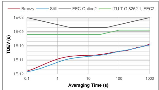
Figure 13. TDEV – Loop Bandwidth 0.1 Hz
