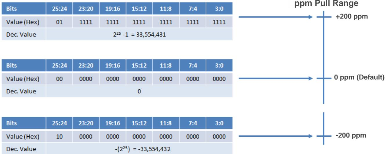
**Figure 31. Pull Range and Frequency Control Word**
