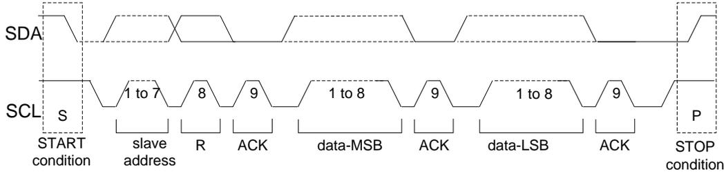
Figure 36. Parallel data byte format, read operation
