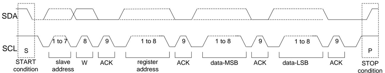
Figure 35. Parallel data byte format, write operation
