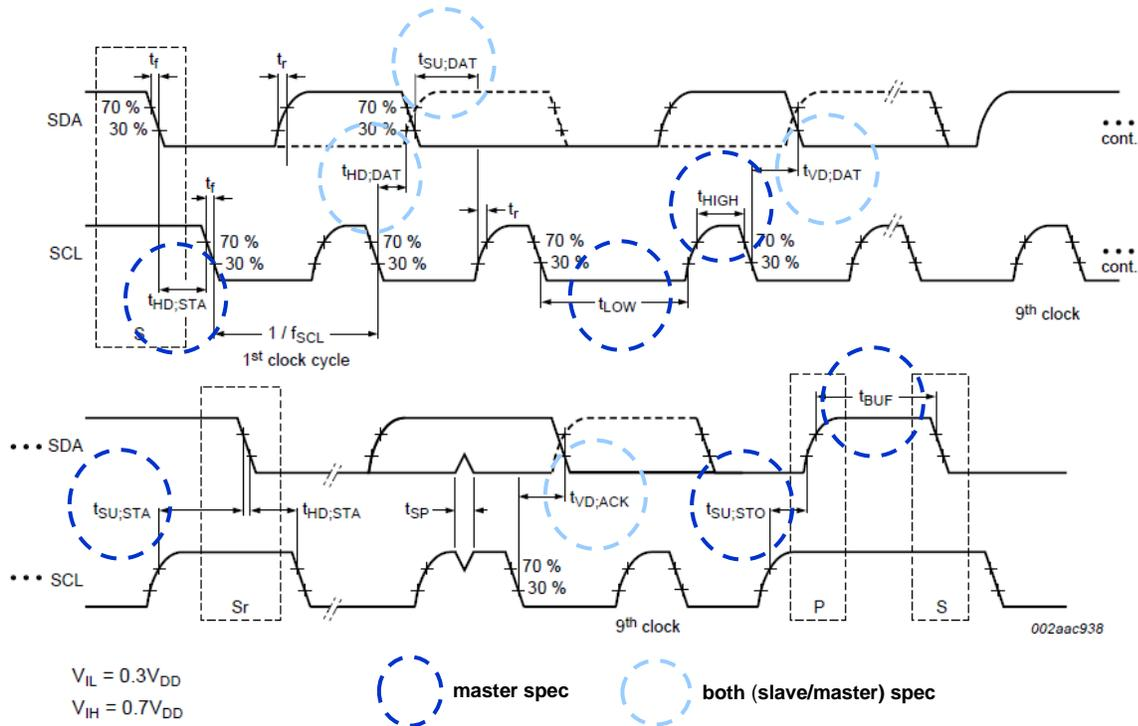
Figure 38. I<sup>2</sup>C Timing Diagram
