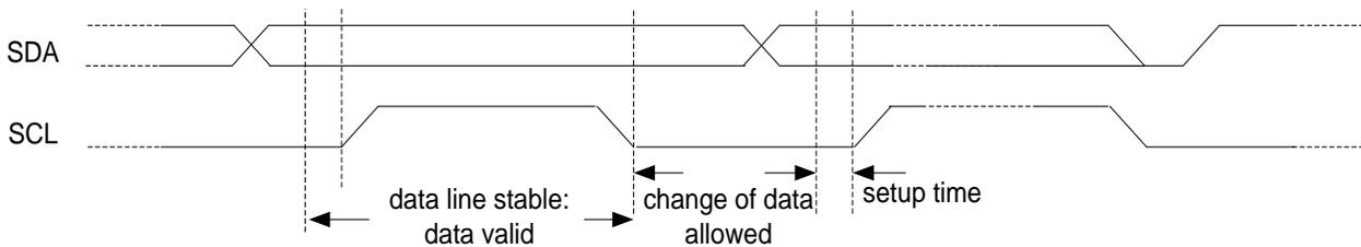
**Figure 32. Data and clock timing relation in I<sup>2</sup>C bus**
