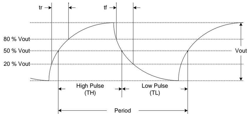
Figure 6. Clipped Sinewave Waveform Diagram<sup>[13]</sup>
