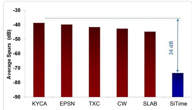
Figure 3. Electro Magnetic Susceptibility (EMS)<sup>[3]</sup>
