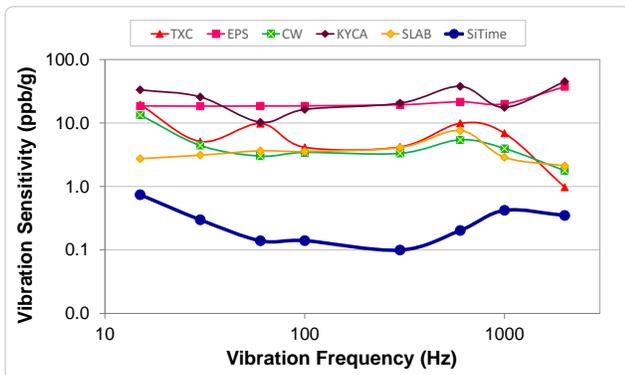
Figure 5. Vibration Robustness<sup>[5]</sup>
