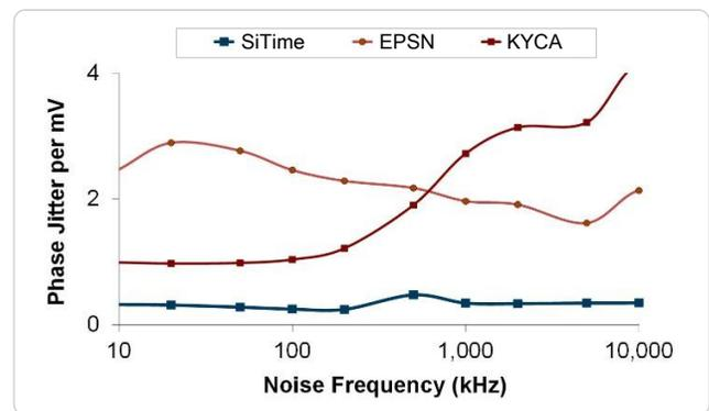
Figure 4. Power Supply Noise Rejection<sup>[4]</sup>
