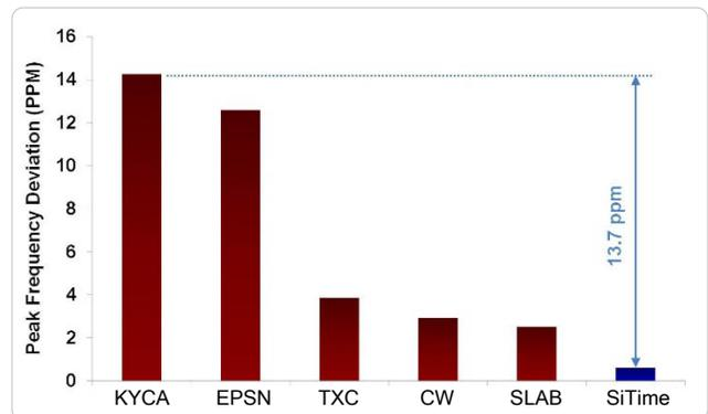
Figure 6. Shock Robustness<sup>[6]</sup>
