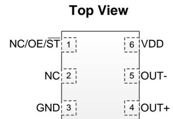
**Figure 1. Pin Assignments**
