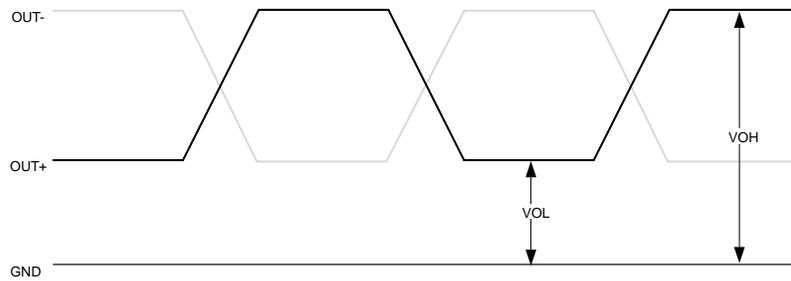
Figure 2. LVPECL/HCSL Voltage Levels per Differential Pin (OUT+/OUT-)
