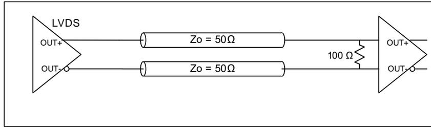
**Figure 12. LVDS single DC termination at the load**
