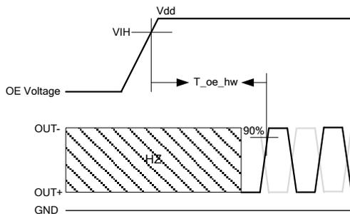
**Figure 6. Hardware OE Enable Timing**
