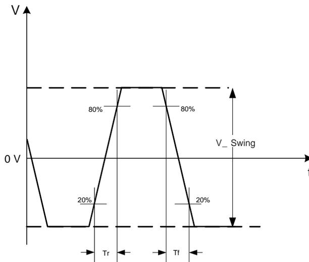
Figure 3. LVPECL/HCSL Voltage Levels across Differential Pair
