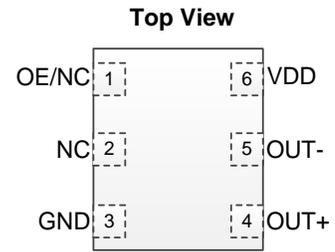
**Figure 1. Pin Assignments**
