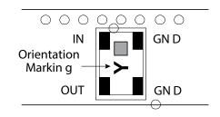
\*The recommended distance to the ground plane is 0.254mm (0.01") \*\* PCB : Taconic Orcer RF-35P
