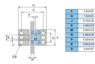
The recommended distance to the PCB Ground Plane is 0.254mm (0.010°) \*\* PCB: Taconic Orcer RF-35P
