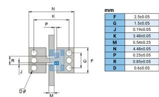
The recommended distance to the PCB Ground Plane is 0.254mm (0.010°) \*\* PCB: Taconic Orcer RF-35P
