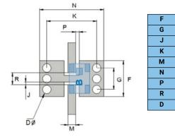
The recommended distance to the PCB  $\,$  Ground Plane is 0.254mm (0.010') \*\* PCB: Taconic Orcer RF-35P  $\,$
