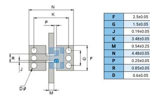
The recommended distance to the PCB Ground Plane is 0.254mm (0.010') \*\* PCB: Taconic Orcer RF-35P
