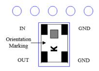
\*The recommended distance to the ground plane is 0.254mm (0.01") \*\* PCB : Taconic Orcer RF-35P
