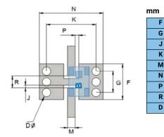
The recommended distance to the PCB  $\,$  Ground Plane is 0.254mm (0.010') \*\* PCB: Taconic Orcer RF-35P  $\,$
