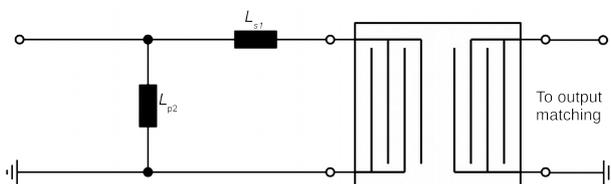
Figure 12: shunt L - series L matching.
