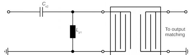
Figure 13: series C - shunt L matching.
