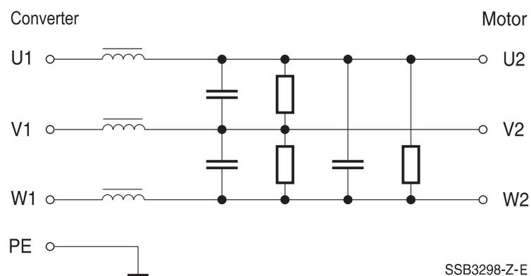
**Sine-wave output filters for 3-phase systems**
